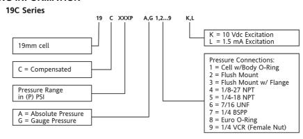
For example: Part #19C100PA4K = 19 mm Cell, Compensated, 100 psi, Absolute, 1/8NPT Port with 10 Vdc excitation.
