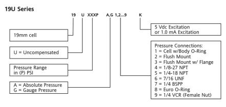
For example: Part #19U100PA4K = 19 mm Cell, Uncompensated, 100 psi, Absolute, 1/8NPT Port with 5 Vdc excitation.
